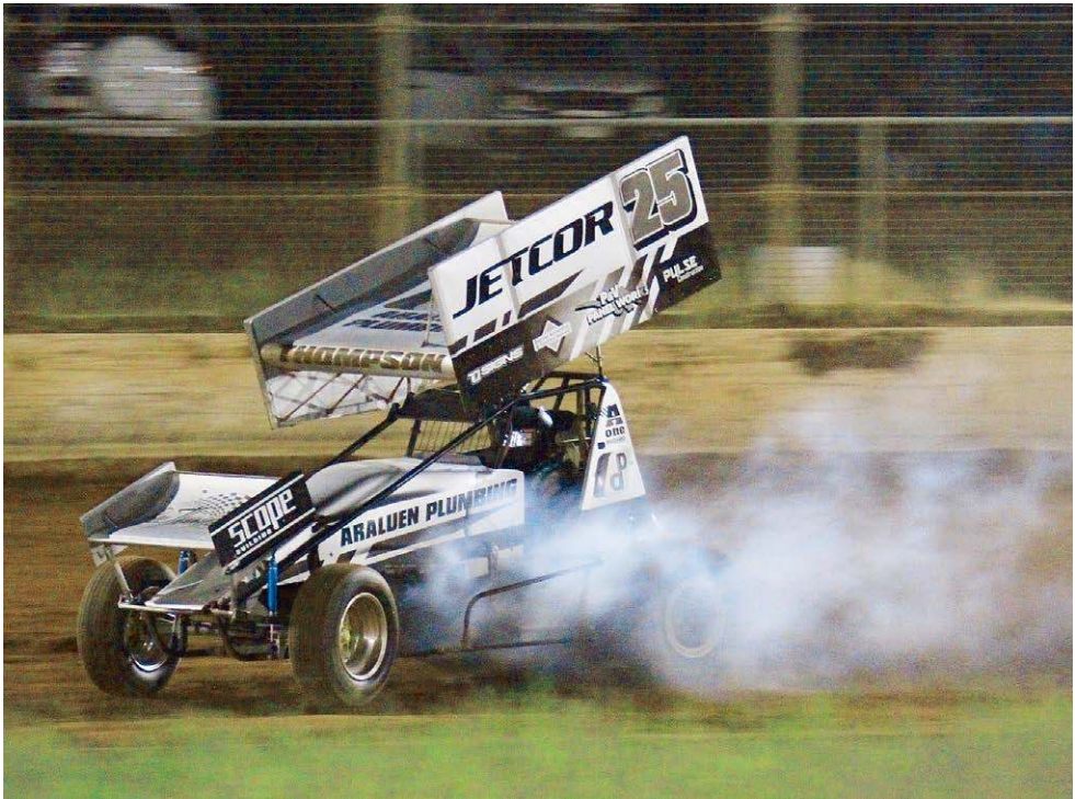
BREATHER: Smoke comes from Warren Thompson's sprint car as oil from a breather pipe hits the hot exhaust. (550977)
