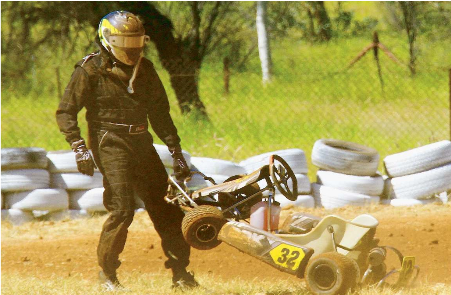
BROKEN: Mark Brownless drags his kart from the track after a blown motor caused him to snap an axel and lose a wheel. (Phil Williams)
